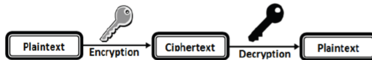
(b) Public-key Cryptography: A pair of keys, one for encryption and the other for decryption.
